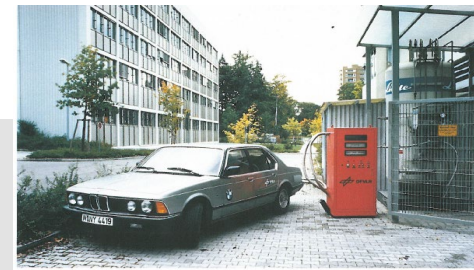
A BMW 745i being tanked at a liquid hydrogen filling station
